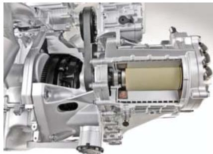
Obr. 11 Rez prevodovkou HDDCT s elektromotorem [8]
