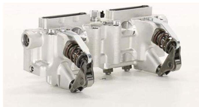
Obr. 16 MultiAir modul motora TwinAir [14]
